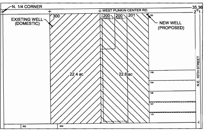
EXISTING DOMESTIC WELL LOCATED 200' SOUTH & 660' EAST OF N 1/4 CORNER OF SECTION 2. PROPOSED IRRIGATION WELL TO BE LOCATED 50' SOUTH & 670' WEST OF NE CORNER OF SECTION 2.
