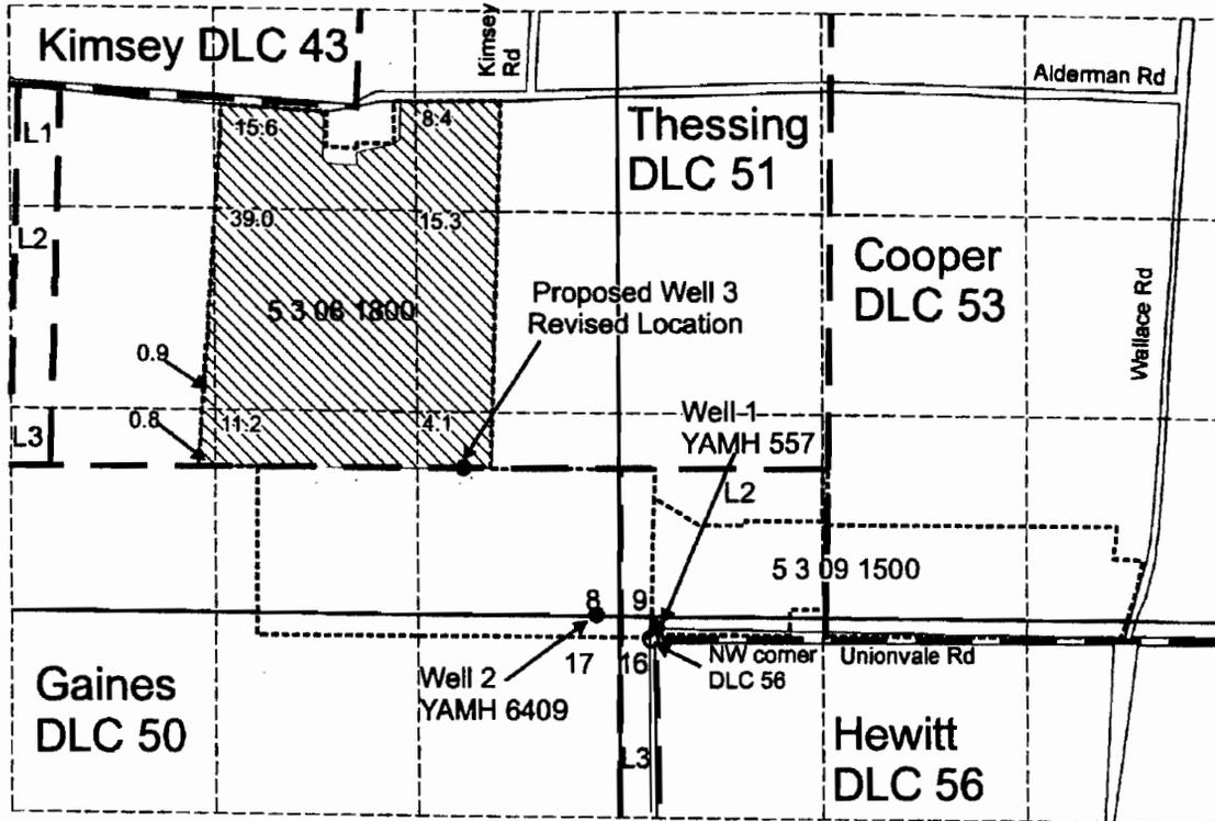
Well 1 (YAMH 557) is located 70 feet north and 5 feet east of the NW corner of DLC 56
