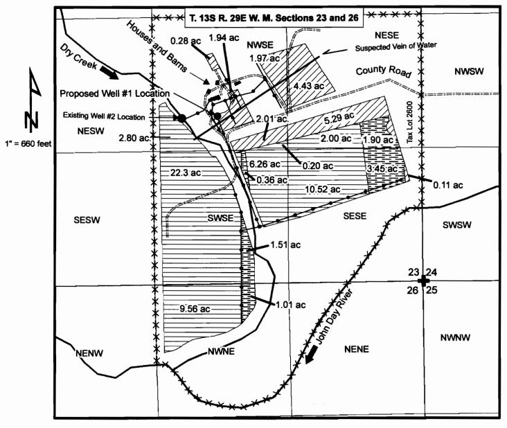
Existing well #2 is located approximately: 1640 feet N and 2360 feet W of SE corner of Sec 23 T. 13S R. 29E W.M.
