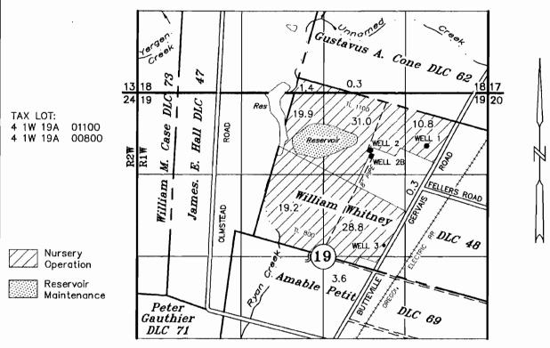
Authorized WELL 1: 1100' S & 2070' E OF THE NW COR OF WILLIAM WHITNEY DLC 48 Authorized WELL 2: 1170' S AND 1170' E OF THE NW COR OF WILLIAM WHITNEY DLC 48 Authorized WELL 3: 185' N AND 1660' W OF THE E 1/4 COR OF SECTION 19
