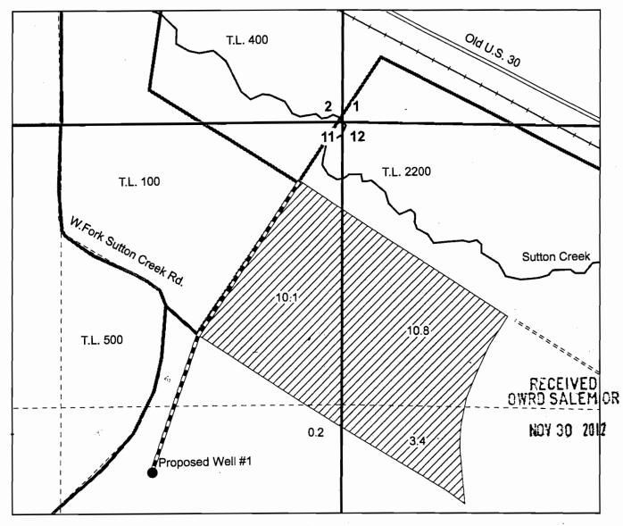
Proposed well #1 is located 1650 feet south and 915 feet west of the NE corner of section 11.
