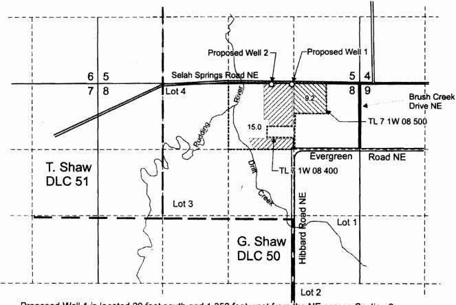
Proposed Well 1 is located 20 feet south and 1,350 feet west from the NE corner, Section 8. Proposed Well 2 is located 20 feet south and 1,750 feet west from the NE corner, Section 8.
