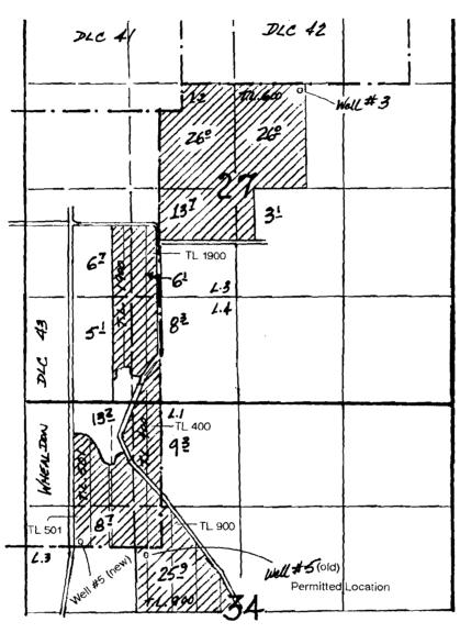
Well #5 (old) was to be located 100' S & 150' W from the SE corner of DLC 43; Permit Amendment to change Well #5 (new) location to: 50' N & 980' W from the SE corner of DLC 43.
