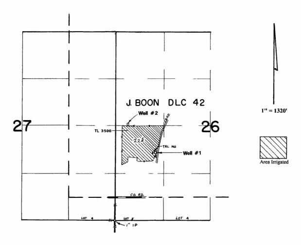
Well #1 is located 1920' N and 1110' E Well #2 is located 2675' N and 352' E-- both from the SW corner of Section 26.
