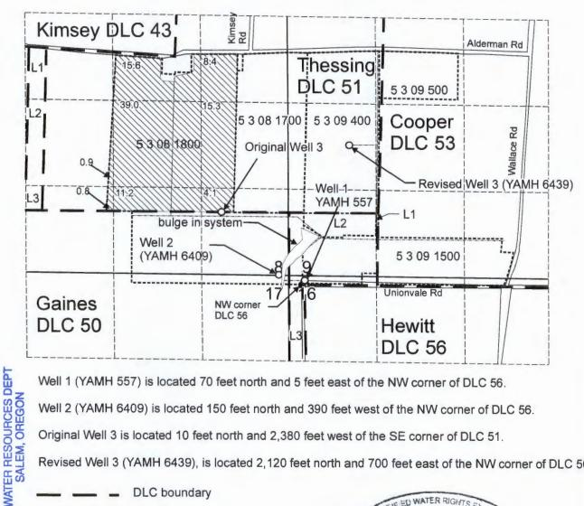
Well 1 (YAMH 557) is located 70 feet north and 5 feet east of the NW corner of DLC 56. Well 2 (YAMH 6409) is located 150 feet north and 390 feet west of the NW corner of DLC 56.
