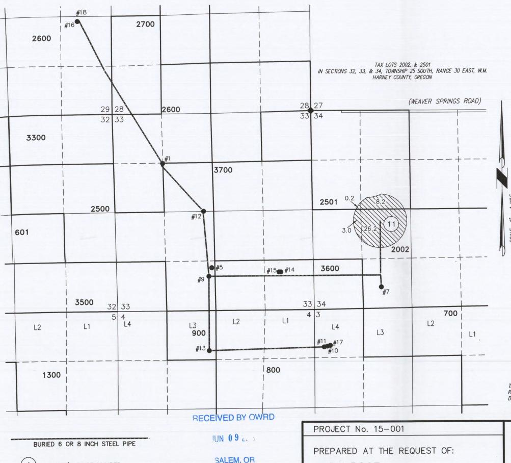
WELL #1 (HARN 1094) PROPOSED 1317' SOUTH & 1355' EAST FROM THE NW CORNER SECTION 33.
