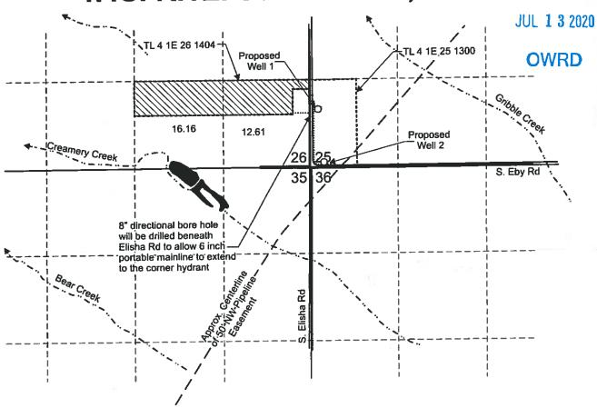
Proposed Well 1 is located 875 feet north and 105 feet east from the SW corner, Section 25. Proposed Well 2 is located 65 feet north and 185 feet east from the SW corner, Section 25.
