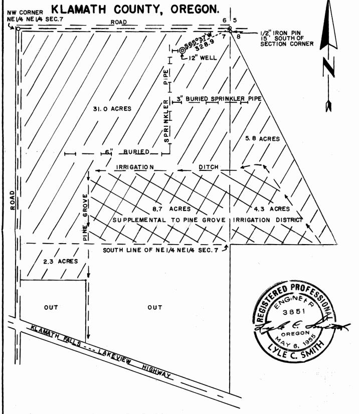
I, LYLE C. SMITH, DO HEREBY CERTIFY THAT THIS MAP WAS MADE FROM NOTES TAKEN DURING AN ACTUAL SURVEY MADE BY ME ON 3-7-58 AND THAT THE MONUMENT SHOWN CONSISTS OF A 1/2" IRON PIN LOCATED 15 FEET SOUTH OF THE NE CORNER OF SECTION 7, T 39S, R 10 EWM.
