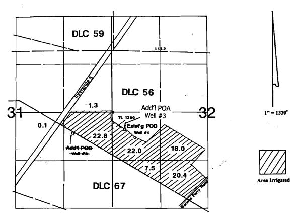
Well #1 is located 690'S & 620'E from the W1/4 corner of Section 32. Well #2 is located 590'S & 1070'W from the W1/4 corner of Section 32.
