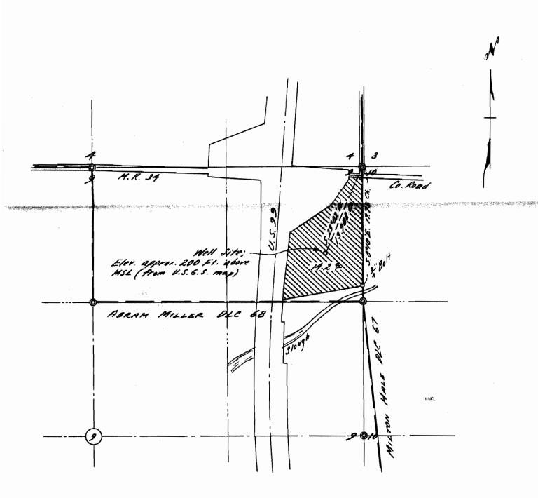
I, Orris A. Carnegie of Albany, Oregon do hereby certify that this map was made from notes taken during an actual survey made by me on October 15, 1957; that the monument shown on this map consisting of a 3/4" iron bolt is S.O°10'E. 17.75 chains from the Northeast corner of Section 9, T. 10 S. R. 3 W. of the Will. Mer. in Linn County, Oregon
