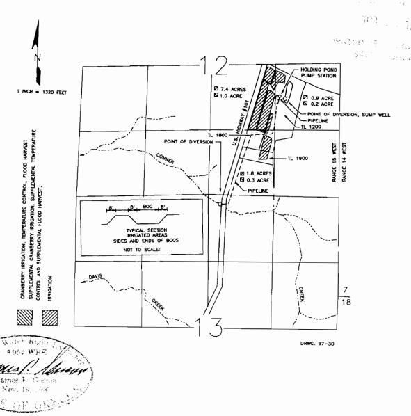
THE SUMP WELL DIVERSION IS LOCATED 1930 FEET NORTH AND 1090 FEET WEST FROM THE SOUTHEAST CORNER OF SECTION 12; BEING WITHIN THE NE1/4 SE1/4 OF SECTION 12; THE CONNER CREEK DIVERSION IS LOCATED 120 FEET SOUTH AND 236) FEET WEST FROM THE SOUTHEAST CORNER OF SECTION 12, BEING WITHIN THE NW1/4 NE1/4 OF SECTION 13, BOTH DIVERSIONS BEING WITHIN TOWNSHIP 30 SOUTH, RANGE 15 WEST, W.M., COOS COUNTY.
