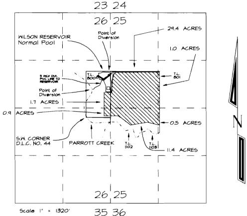
Point of Diversion from Milson Reservoir is 1166 feet North and 628 feet East of the S.M. Corner D.L.C. No. 44
