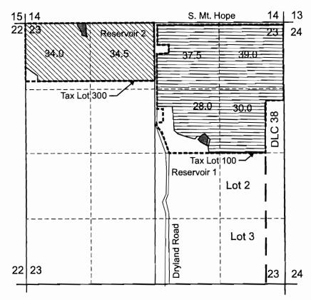
Reservoir 1 is located 2,370 ft S. And 1,660 ft. W. from the NE corner, Section 23. Reservoir 2 is located 100 ft. S. And 1,150 ft E. from the NW corner, Section 23
