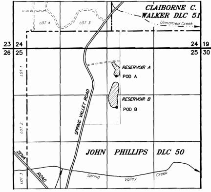
POD A: 1275' S & 135' E OF THE SW CORNER CLAIBORNE C. WALKER DLC 51 POD B: 2160' S & 145' E OF THE SW CORNER CLAIBORNE C. WALKER DLC 51
