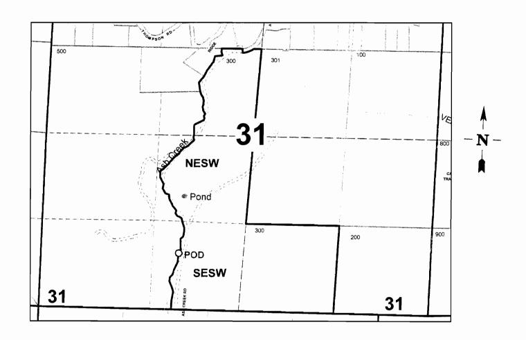
Pond is 2200 ft. S. and 2300 ft. W. from the NE 1/16 corner of section 31. POD is 3155 ft. S. and 2333 ft. W. from the NE 1/16 corner of section 31.
