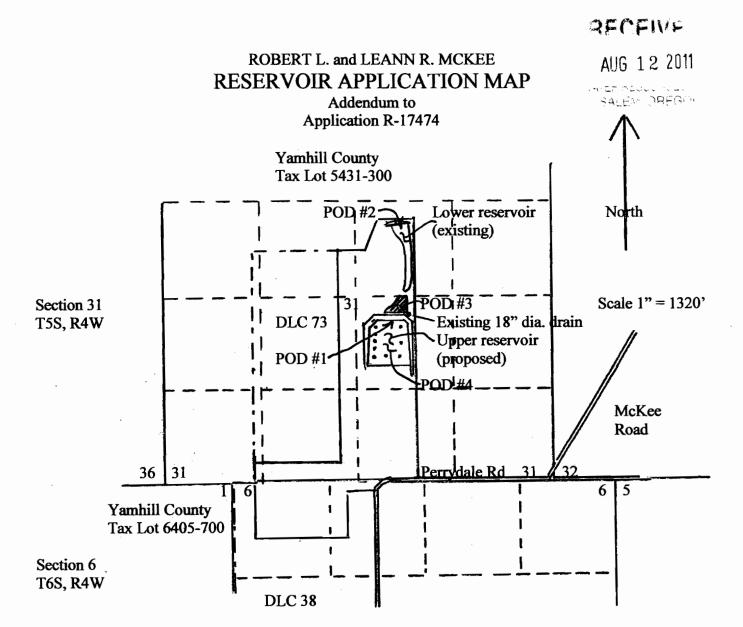
POD #1 for upper reservoir is located 400' east and 350' south from the center of Section 31, T5S, R4W POD #2 for lower reservoir is located 550' east and 1000' north from the center of Section 31, T5S, R4W (existing reservoir P-77020)
