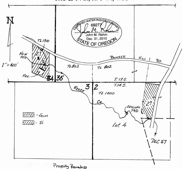
POD's Located: Original POD- 530' S. & 580' E.; New POD- 310' N. & 810' W.; Reservoir- 220' N. & 850' W; all from the NW Corner, Section 2, T. 14 S., R. 6 W.
