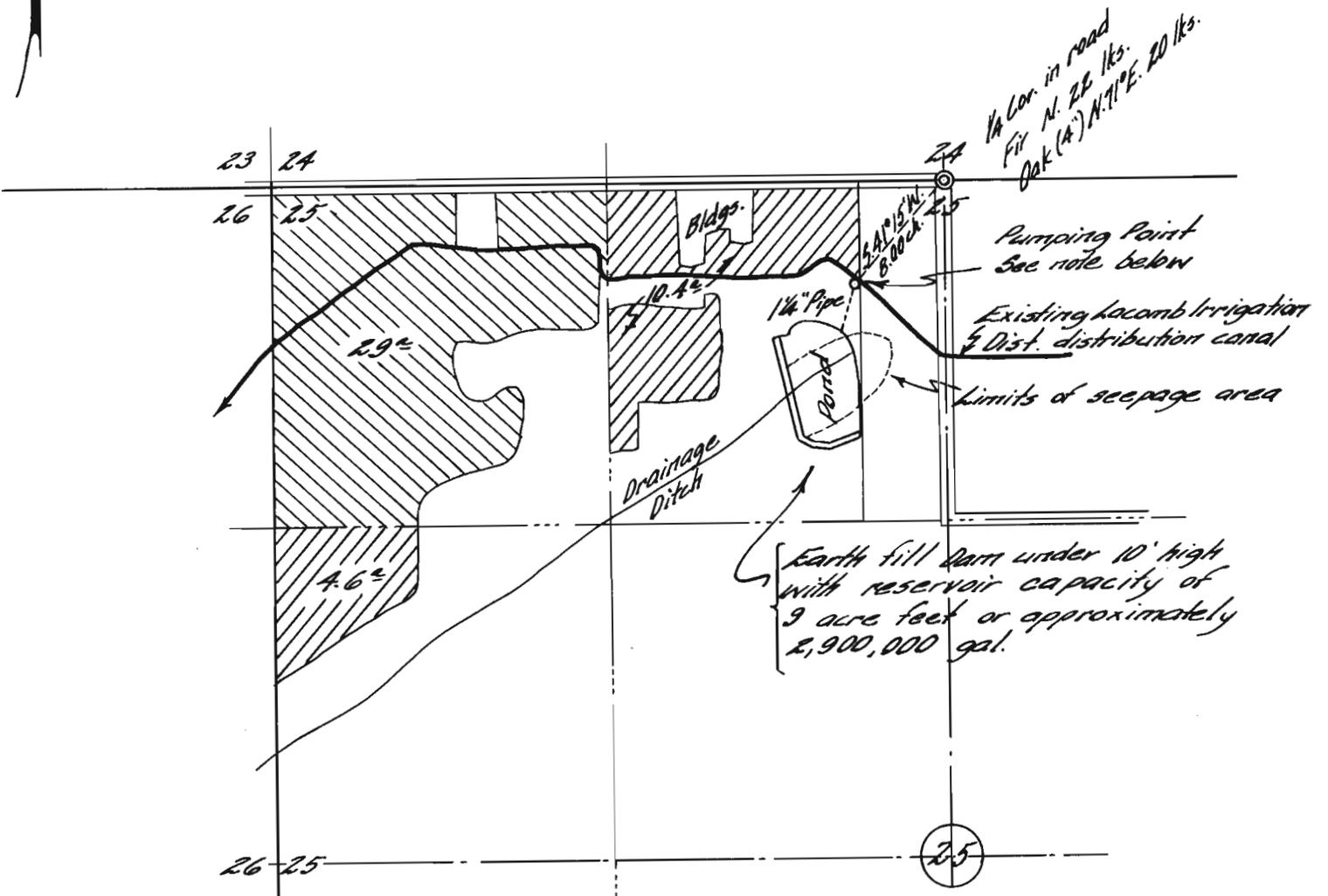
*Note: Present plan is to use the existing Lacomb Irrigation ditch as distribution ditch by pumping from pond into said ditch, a lift of only about 3 1/2 feet, then flood irrigating where possible from the ditch and using sprinklers, where impossible to flood irrigate, by portable pumping along the ditch. It is also planned to use some water from the present canal, during slack periods, to keep up the level of the pond by ditching from canal to pond near the pumping point.*
