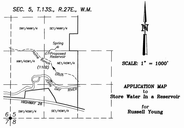
Approximate center of proposed reservoir is 2570 ft. North and 1450 ft. East of the Southwest Corner of Section 5, T.13S., R.27E., W.M.
