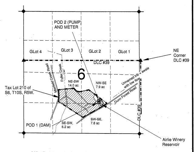
POD 1 (Dam) (west edge of rservoir) is 1420' N & 1840' W and POD 2 (Pump) (NW of reservoir) is 1490' N & 1860' W of SE S6.
