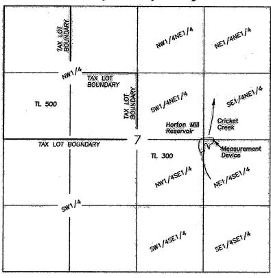
Outlet is located 2620' North & 1100' West of the SE corner of Section 7. Measuring device is located 5' West of the Outlet
