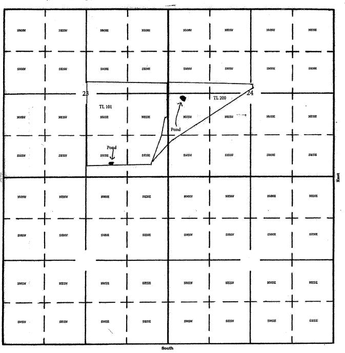
Dam: 405 North & 1725 West from SE Corner Section 23 Dam: 2,400 North & 525 East from SW Corner Section 24
