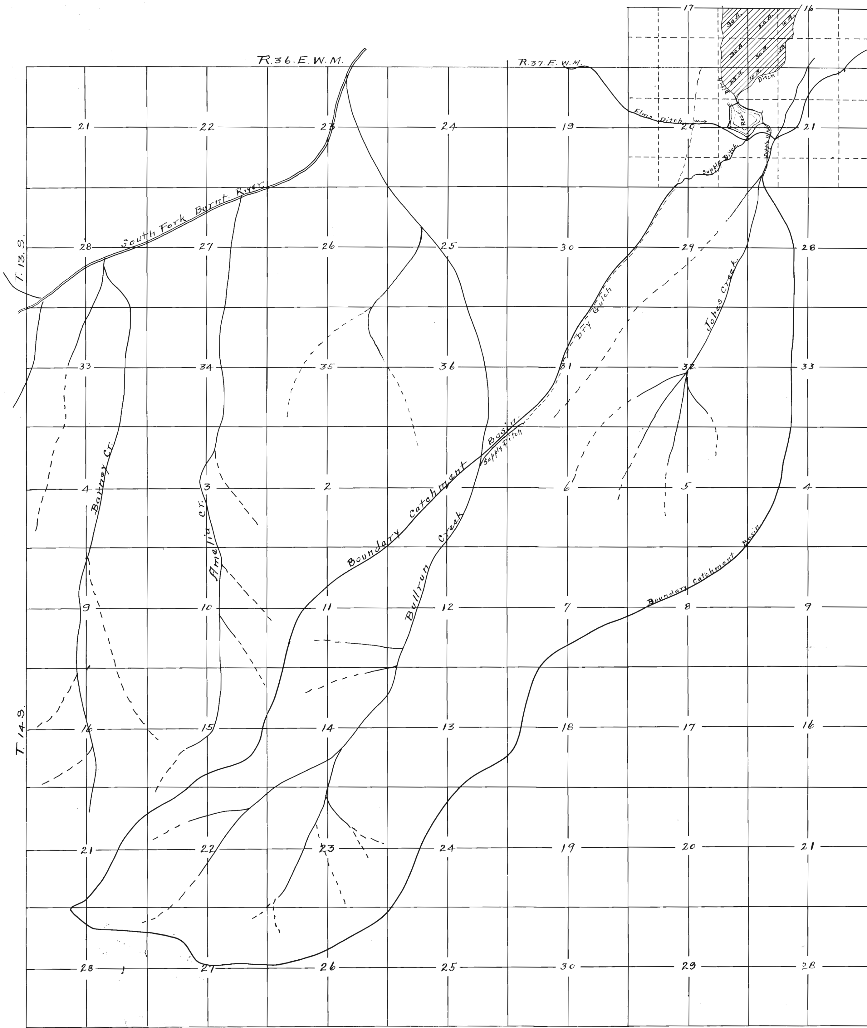
Map Showing the location of Mortitt Reservoir, Catchment Basin, and Land to be Irrigated. Scale - 2 inches = 1 mile.
