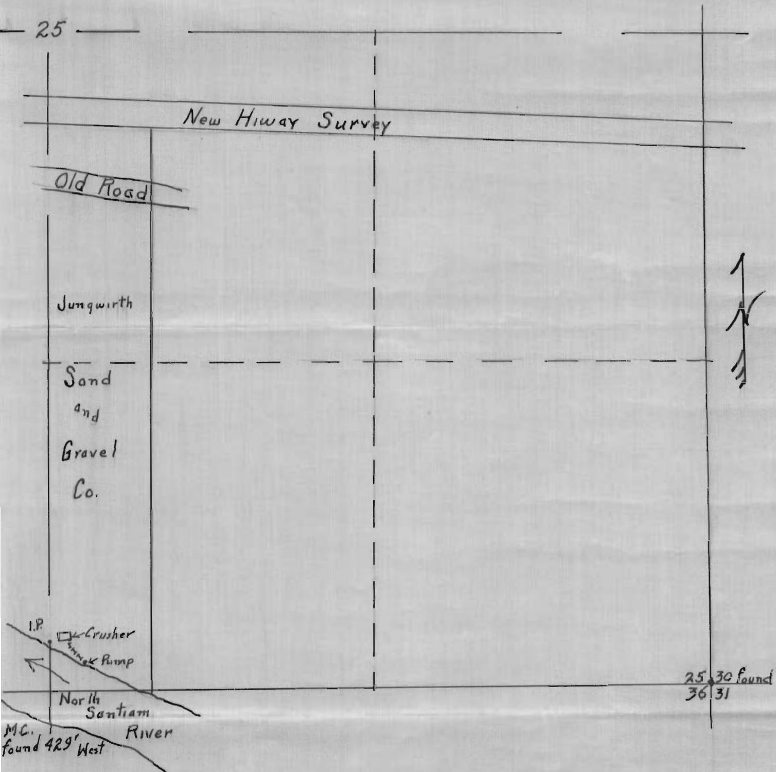
I, L Burl Smith of Lyons Ore. do hereby certify that this map was made from notes taken during an actual survey made by me on April 9, 1949; that the monument shown on the map is a 1" iron pipe 36" long - 30 inches in the ground - 190 ft North of  $\frac{1}{4}$  corner between Sec's. 25 & 36 T. 9. S., R. 2. E. W.M.
