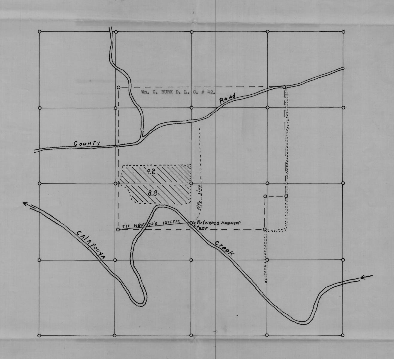
I, WILFORD N. HAINES of DRAIN OREGON do hereby certify that this map was made from notes taken during an actual survey made by me on April 3, 1952; that the monument shown on this map consisting of a 1½" iron pipe 36" long driven 30" in the groun is N. 84° 50' E. 1224.6 ft. from the SW.Cor. of the Wn. C. BURK D. L. C. # 42.
