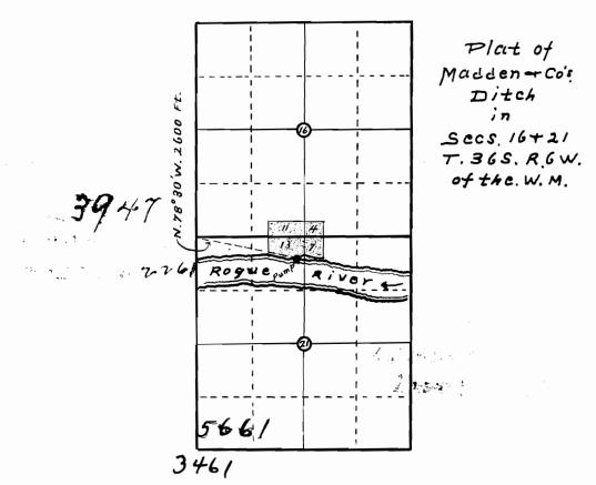
I, Horace C. Hall, of Grants Pass, Oregon, do hereby certify that this map was made from notes taken during an actual survey made by me on the 8th day of September, 1914, and that it correctly represents the works described in the accompanying application, together with the location of streams and other ditches in the immediate vicinity, and has written thereon the area in each smallest legal subdivision which it is proposed to irrigate.
