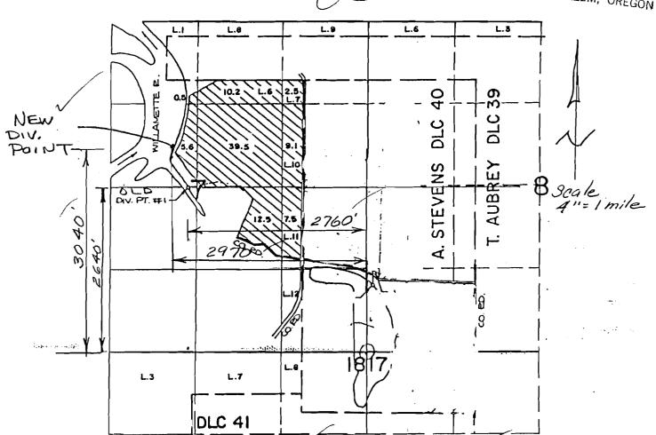
OLD DIV POINT IS LOCATED 2640 FEET NORTH AND 2760 FEET WEST FROM THE SW CORNER OF SECTION 8 OF THE WILLAMETTE MERIDIAN. NEW DIV. POINT WILL BE LOCATED 2970 FEET WEST AND 3040 FEET NORTH OF SAID SW SECTION CORNER.
