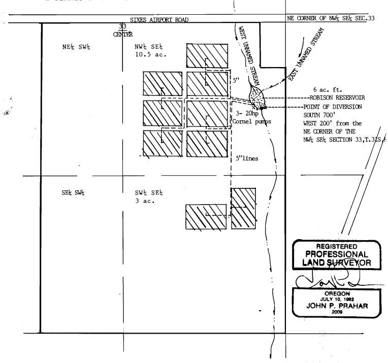
MAP FOR APPLICATION TO APPROPRIATE SURFACE WATER AND CONSTRUCT A RESERVOIR
