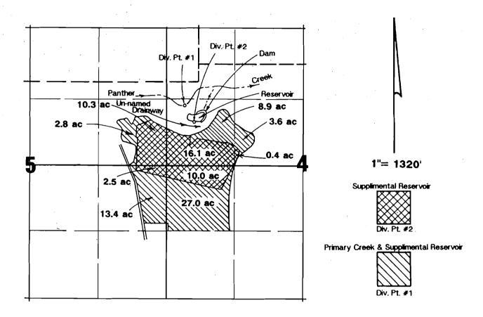
Dam located 1070'N & 750'E from SW cor. NW1/4 Section 4. Div. Pt. #1 located 1200'N & 370'E from SW cor. NW1/4 Section 4. Div. Pt. #2 located 880'N & 540'E from SW cor. NW1/4 Section 4.
