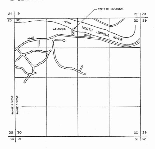
THE POINT OF DIVERSION IS TO BE LOCATED 500 FEET SOUTH AND 190 FEET WEST FROM THE NORTH 1/4 CORNER OF SECTION 30, BEING WITHIN THE NE 1/4 OF THE NW 1/4 OF SECTION 30, TOWNSHIP 26 SOUTH, RANGE 5 WEST, W.M., DOUGLAS COUNTY.
