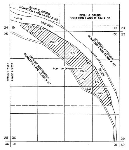
THE POINT OF DIVERSION IS TO BE LOCATED 1380 FEET SOUTH AND 1400 FEET WEST FROM THE NORTHEAST CORNER OF SECTION 30, BEING WITHIN THE SW 1/4 OF THE NE 1/4 OF SECTION 30, TOWNSHIP 26 SOUTH, RANGE 6 WEST, W.M., DOUGLAS COUNTY.
