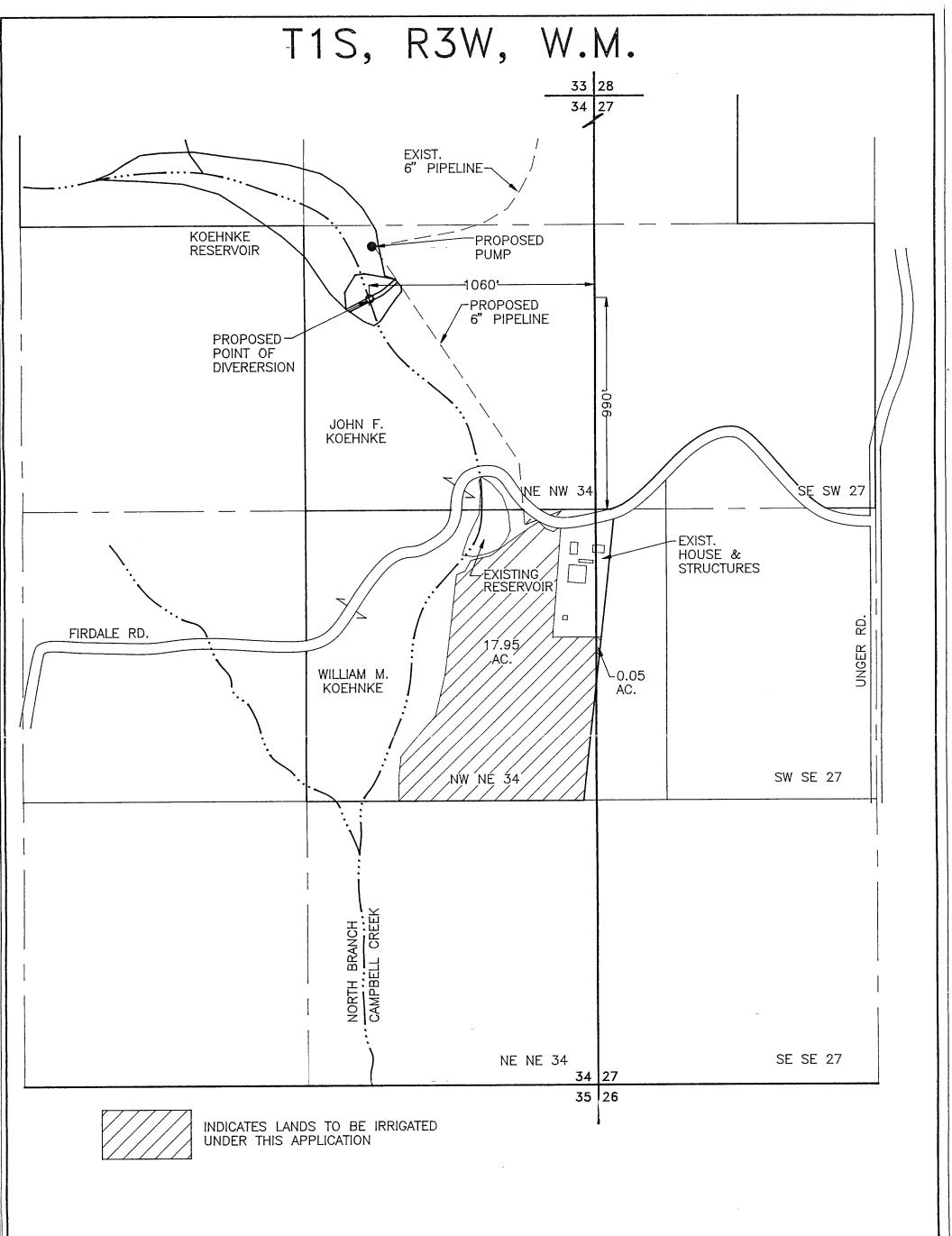
MAP TO ACCOMPANY APPLICATION FOR A PERMIT TO APPROPRIATE SURFACE WATER FOR JOHN F. KOEHNKE SECTIONS 27, 34, T1S, R3W, W.M. WASHINGTON COUNTY, OREGON
