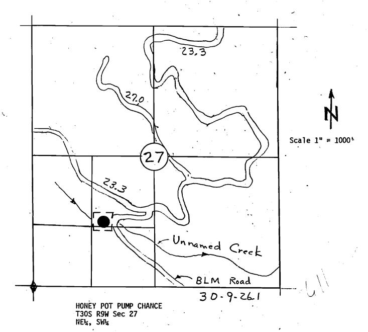
The point of diversion is located 1350 ft North and 1400 ft East from the Southwest Section corner of Section 27.
