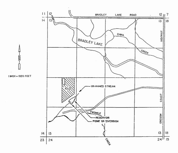
THE POINT OF DIVERSION IS TO BE LOCATED 3770 FEET SOUTH AND 4150 FEET WEST FROM THE NORTHEAST CORNER OF SECTION 13, BEING WITHIN THE NW 1/4 OF THE SW 1/4 OF SECTION 13, TOWNSHIP 29 SOUTH, RANGE 15 WEST, W.M., COOS COUNTY.
