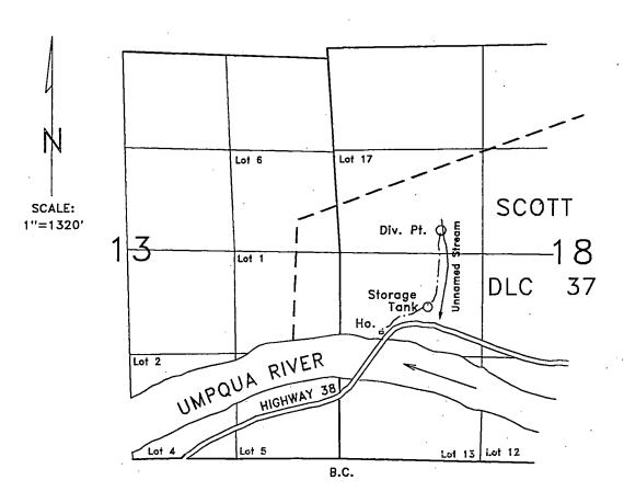
Div. Pt. is located 2800' N. & 1250' E. from SW corner of Section 18.
