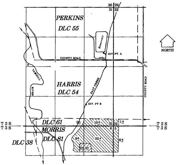
DIV. PT. A: 250' North and 1500' West of the SE corner of the Perkins DLC No. 55 DIV. PT. B: 1960' South and 2260' West of the SE corner of the Perkins DLC No. 55
