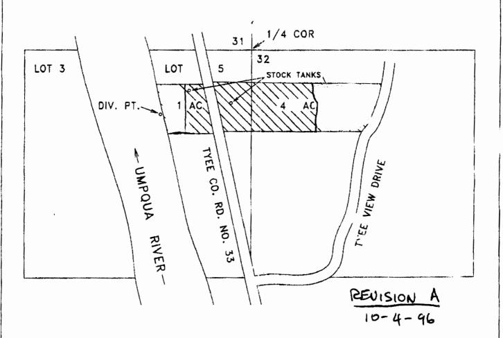
THE DIVERSION POINT IS LOCATED 380 FEET SOUTH AND 535 FEET WEST FROM THE EAST 1/4 CORNER OF SECTION 31, BEING WITHIN GOVERNMENT LOT 5 (NE 1/4 OF THE SE 1/4) OF SECTION 31, T 24 S, R 7 W, W M.
