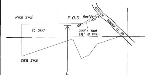
The P.O.D. will be an inspring screened tile with 200+ feet of 1½ inch diameter PVC connecting to the place of use. The P.O.D. will be located 656 feet West and 1477 feet North from the West 1/16 corner of Section 17.
