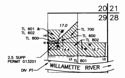
DIV PT: SOUTH 780 FT & EAST 60 FT FROM 1/16 CORNER SECTION 29, T11S, R4W, W.M. IN THE SW1/4 NE1/4 (LOT 3) SECTION 29.
