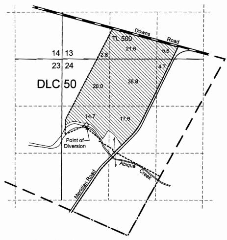
Point of Diversion is located 800 feet north and 700 feet east from the W 1/4 corner of Section 24.
