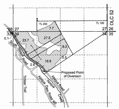
Proposed Point of Diversion is located 2,220 feet south and 1,610 feet east from the NW corner, Section 34.
