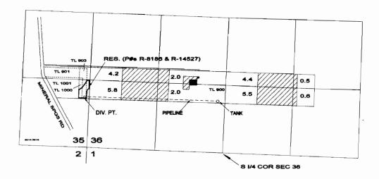
THE DIV. PT. IS LOCATED 980 FT N AND 50 FT W FROM THE S 1/4 CORNER OF SECTION 36
