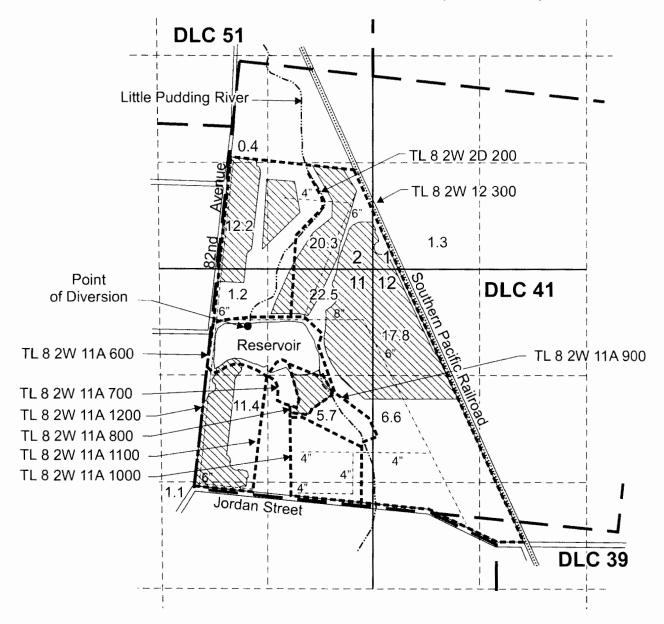
Proposed point of diversion is located 690 feet S. and 1,070 feet E. from the N 1/4 corner of Section 11.
