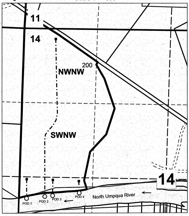
Point of Diversion 1 is 380' South and 140' East Point of Diversion 2 is 375' South and 460' East Point of Diversion 3 is 370' South and 600' East Point of Diversion 4 is 325' South and 1070' East all from the West 1/4 Section Corner.
