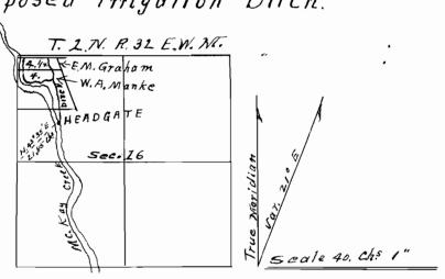
I. W. Kimbrell of Pendleton Or. do hereby certify that this map was made from notes taken during an actual survey made by me on the 30th day of April 1911 and That it correctly represents. The Location of The Proposed Headgate, and ditch, and has written Thereon the area in each smallest Legal Subdivision. Which it is Proposed to Irrigate.
