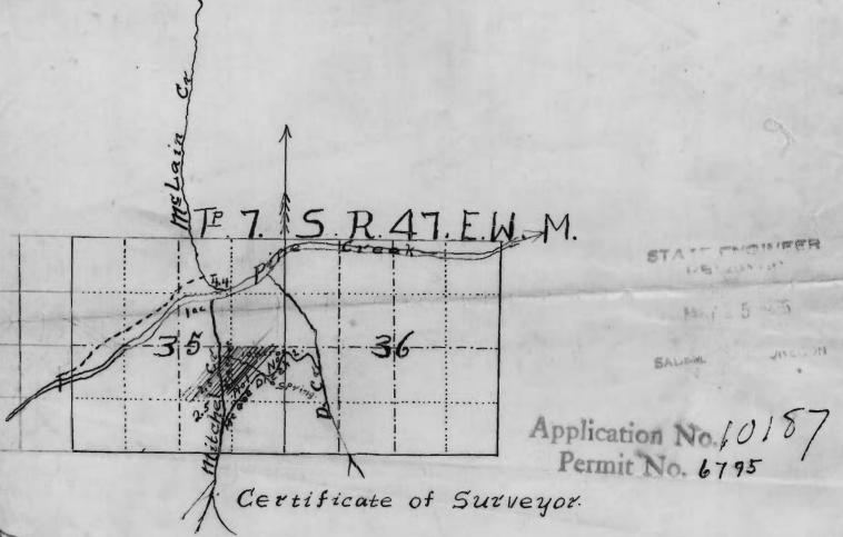
1.W.BBlakeslee of Halfway Oregon do hereby certify that this map was made from notes taken during an actual Survey. made by me on April 21st 1915 and that it correctly represents the works described in the accompanying application togather with the location of Streams and othe ditches in the immediate vicinity, and has written thereon the area in each smallest legal subdivision which it is proposed to irrigate,
